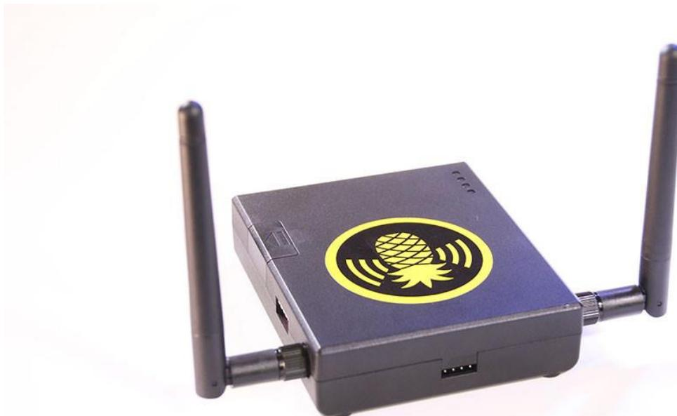
Slika 3 – WiFi Pineapple Mark V – penetration testing WiFi Access Point
